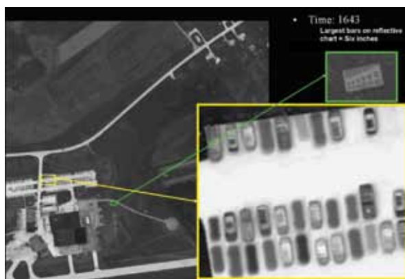
FIGURE 8 DB-WAPSS daytime MWIR flight imagery (June 9, 2009). Inset images show (top) a resolution target, and (bottom) vehicles in a magnified view of the parking area.
