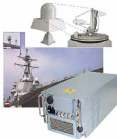
A high-performance, hardware-in-the-loop simulator for real-time closed-loop testing and evaluation of electronic warfare systems and techniques to counter the antiship missile threats.
