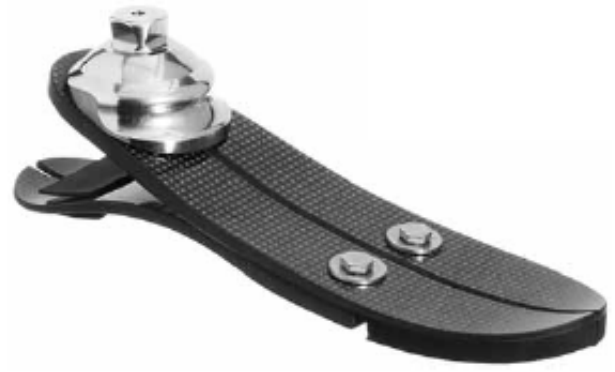
Fig. 5. The low profile of the LP Vari-Flex foot by Ossur provides a low clearance keel and opens up room for a more complicated joint above it. The portion of the keel that low-profile version removes is not needed in a device with an active ankle joint, as its only purpose is to add flexibility of the ankle in a passive prosthesis.
