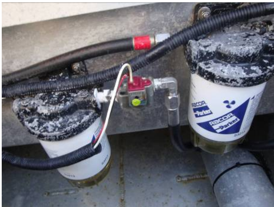
Figure 3. FloScan meter currently installed on all RB-S platforms.
