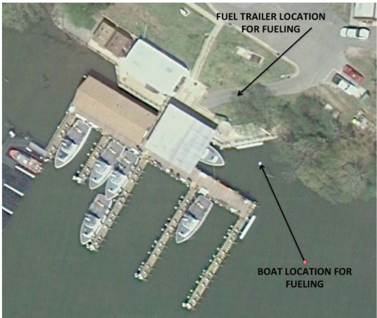
Figure 9. Location of fuel trailer during refueling.
