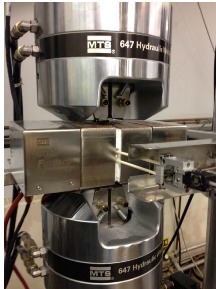
Figure 11: Test assembly showing the MTS 653 furnace and the Extensometer
