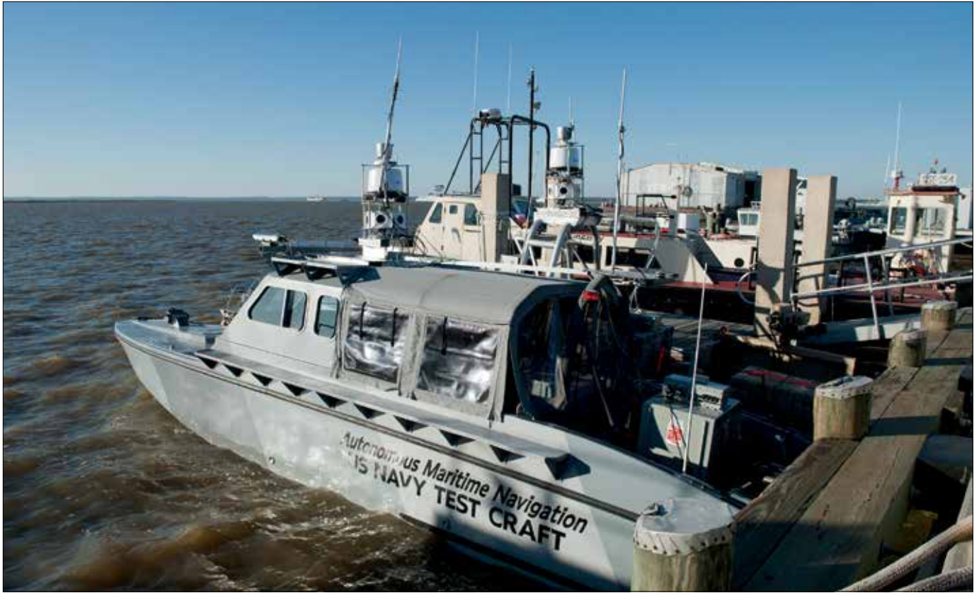
U.S. Navy unmanned surface vessel is equipped with cameras, computer systems, and nonlethal weapons during Trident Warrior (U.S. Navy/Betsy Knapper)
