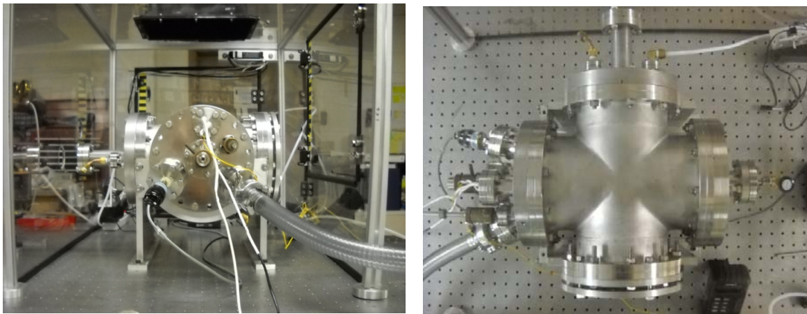
Figure 47: Laser-Assisted Spray deposition system for the fabrication of hybrid structures.
