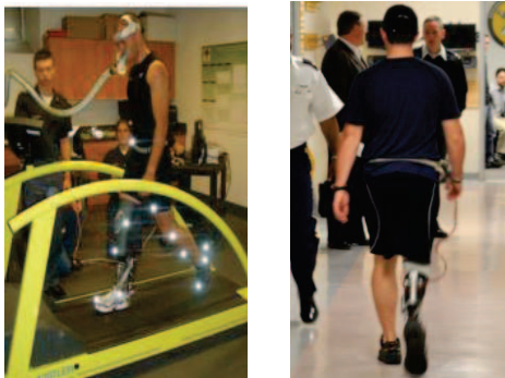
Fig. 3. Transtibial amputee subjects during metabolic and gait studies using two of the newer prototypes.
