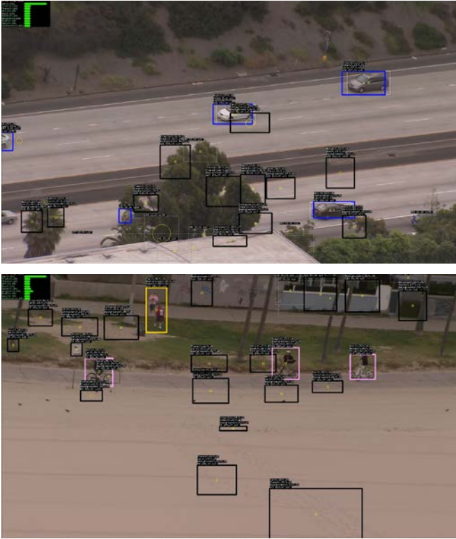
Fig. 6. Examples of detections with the USC algorithm on Heli clips. Black boxes have been attended to but classified as background and are eliminated from final output. Blue: cars; Yellow: humans; Pink: bicycles.
