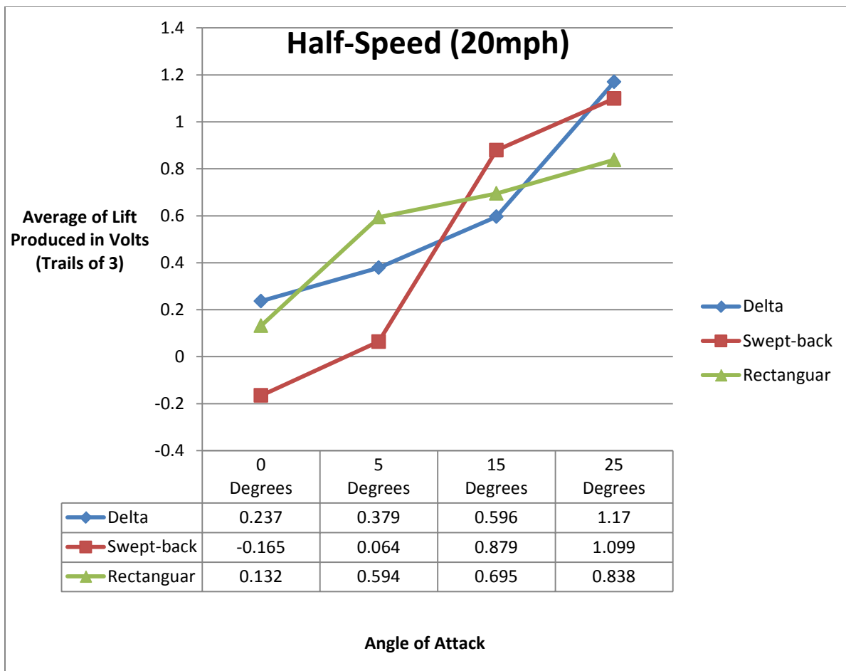
Figure H-21 Half-speed Lift Produced by Wings
