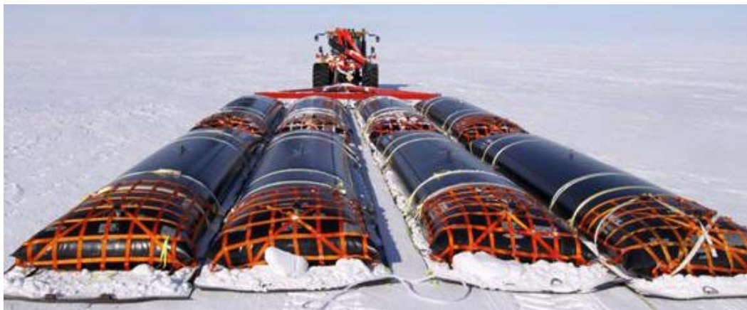
Figure 1. Fuel sleds towed outbound from McMurdo Station to South Pole Station in 2010–11. Each 8 ft wide \times 68 ft long \times 0.5 in. thick HMW-PE sheet carries two 3000 gal. fuel bladders.
