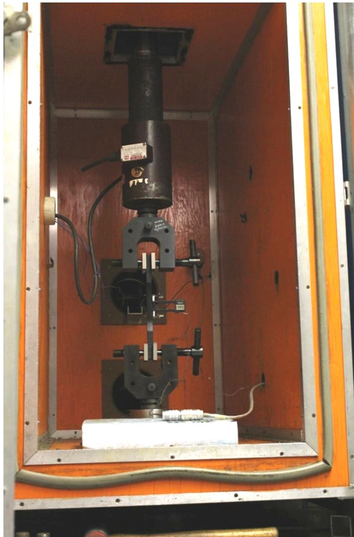
Figure 3. HMW-PE specimen ready for tensile testing inside environmental chamber.
