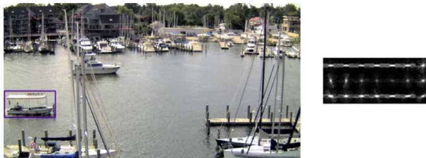
Figure 1. In this image, the water taxi surrounded by the bounding box is taken as a positive instance for the water_taxi category (left). The confined area is extracted and converted to a HOG feature set for training (right).
