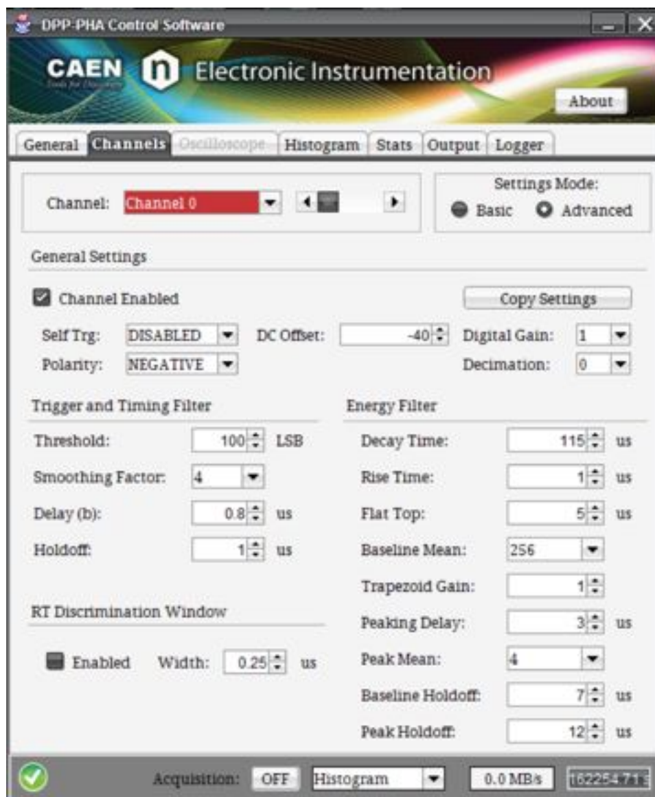
Figure 29. Computer software settings for pulse height analysis of the NaI(Tl) detectors.
