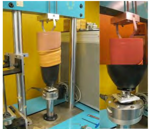
Figure 5 Experimental setup for simulated static loading of the limb phantom/socket system.
