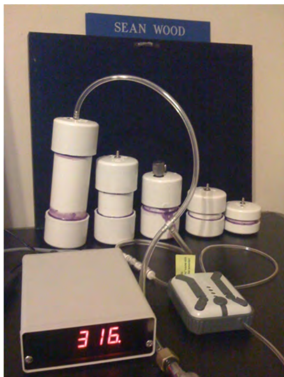
Figure 5: The test setup used for bench-top testing with the 5 test canisters in the back, digital vacuum gauge at front left and e-Pulse vacuum pump at front right.
