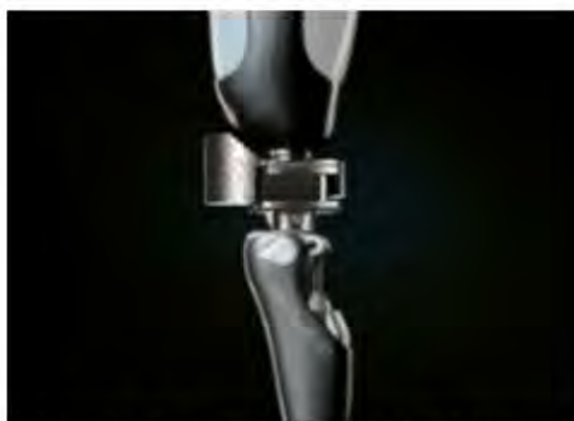
Figure 16: An artists' rendering of the hybrid pump mounted between a socket and C-Leg.
