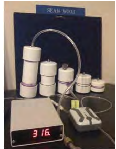
Figure 9 The test setup used for bench-top testing with the five test canisters in the back, digital vacuum gauge at front left and e-pulse vacuum pump at front right.
