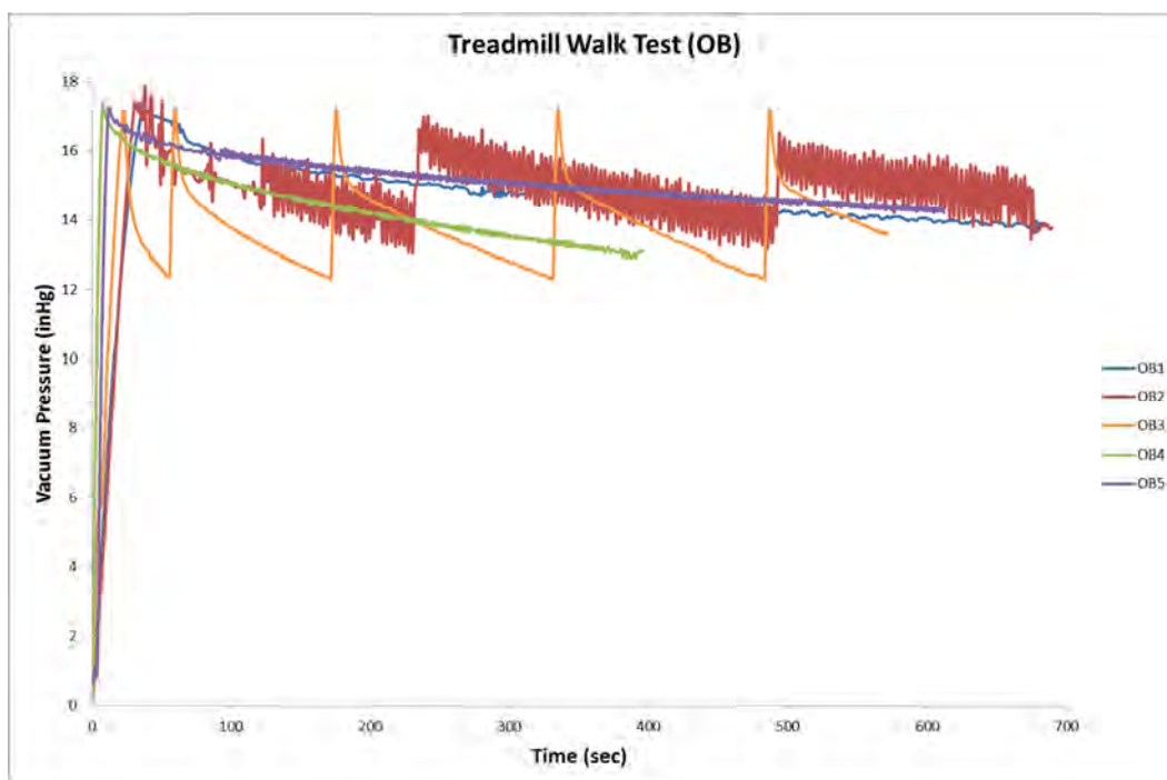
Figure 13: Vacuum pressure over time recorded during treadmill testing using the e-Pulse
