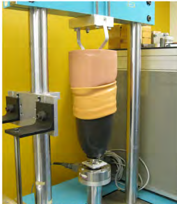
Figure 2: The limb phantom and socket system setup in the mechanical testing device
