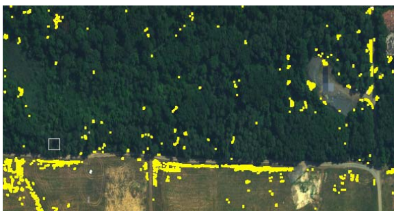
Figure 3 - Application of Target Detection Algorithms Searching for Green Panels [Image on left demonstrates multiple false alarms using direct spectral matching technique. Image on right demonstrates accurate detection of concealed panels using Invariant Algorithm]
