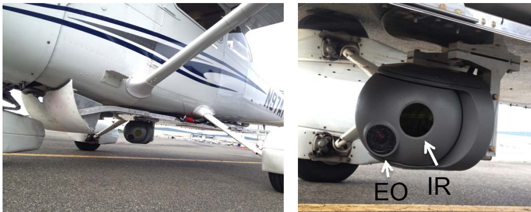
Figure 2. ( left ) The gimbal as is mounted on the belly platform of the Cessna 172 survey plane. ( right ) A close-up of the gimbal showing the windows for the visual (EO) and the mid-wave thermal (IR) cameras. Cabling into the cabin for the data output, serial control and power are not visible in the picture.
