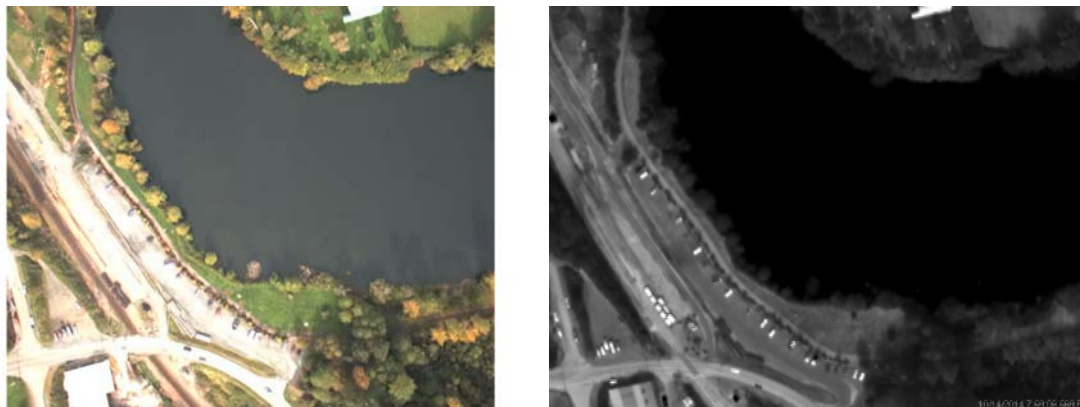
Figure 3. ( left ) Visual band image, and ( right ) thermal IR band image from a bend in the Snohomish River near Everett WA. Cooler brightness temperatures, including the relatively cold river, are displayed as low (dark) intensities.
