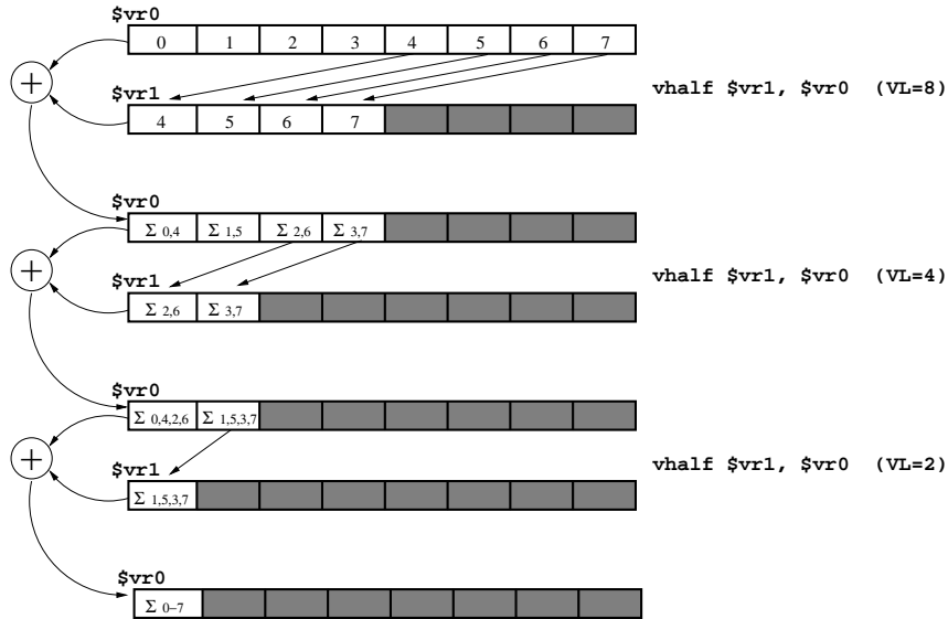
Figure 4.3: An add reduction of a vector with eight elements using the vhalf permutation instruction. The instruction reads the second half of the source register and copies the elements at the beginning of the destination register. The vector length register, which must be a power of two, indicates the number of elements in the register at any time. A reduction step consists of vhalf followed by a vector addition of the source and destination registers of the permutation at half the vector length. Three iterative steps are necessary to reduce the initial vector to a single element value.
