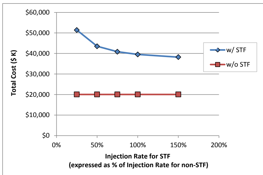
Figure 23. Sensitivity of cost of shear-thinning technology to injection rate. (Scenario 1: single injection)
