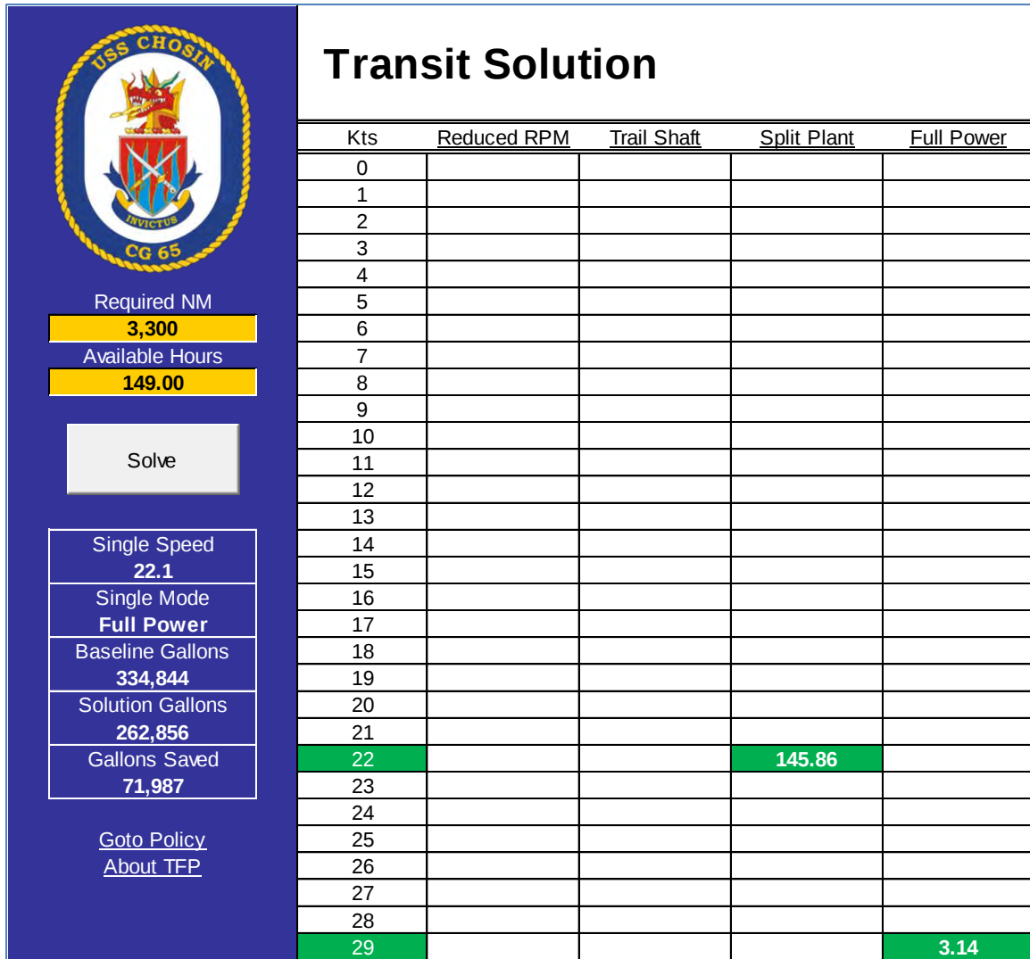
Figure 10. Utilizing the TFP for a 3,300 nm transit completed in 149 hours can reduce fuel consumption by 71,987 gallons, which is a 21% savings.
