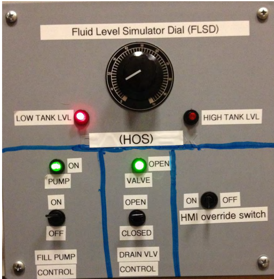
Figure 5. HMI Override Station front panel including FLSD
