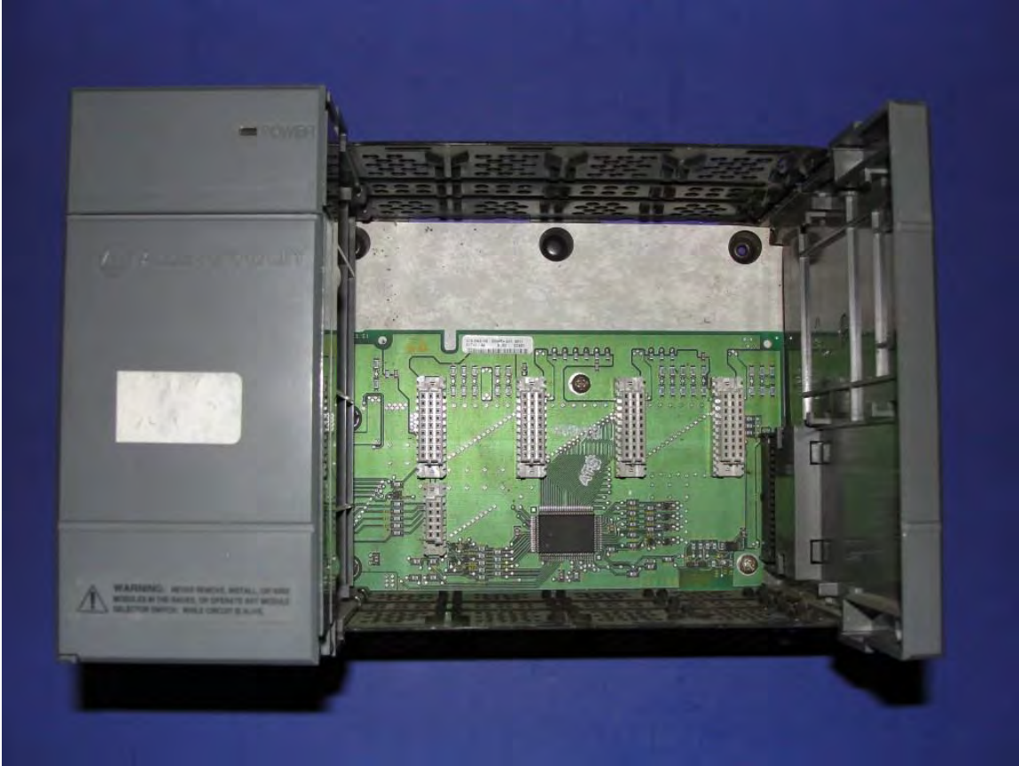
Figure 4. Allen Bradley 1746-A4 (4-slot I/O chassis) with power supply
