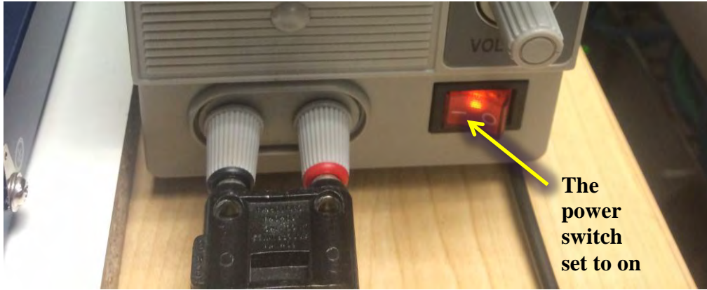
Figure F13a. Variable DC power supply powered ON only
