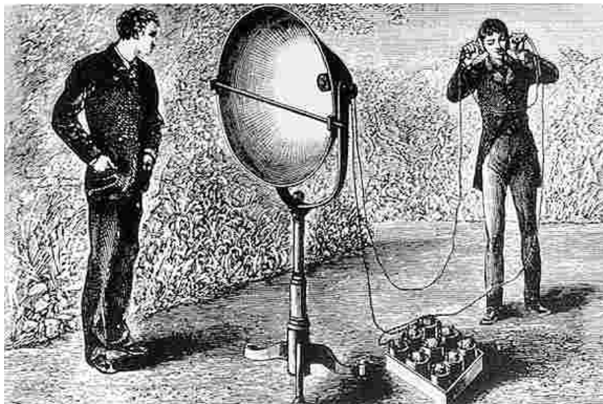
Figure 2. A photophone receiver, from [12].
