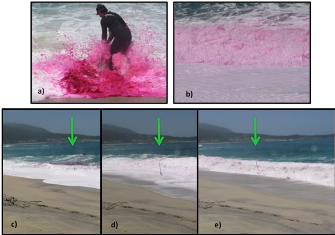
Figure 32. Photos showing examples of (a) the initial dye slug release, (b) the well-mixed surf/swash zone shortly after the dye release, and (c-e) a dye sensor attached near the sea-bed on a pole (shown by the green arrows) in the surf zone, highlighting the intermittency of the dye observations as the sensor is alternately submerged and not submerged.
