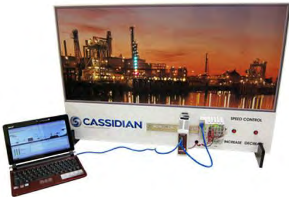
Figure 8. Tofino SCADA Security Simulator, from [16]
