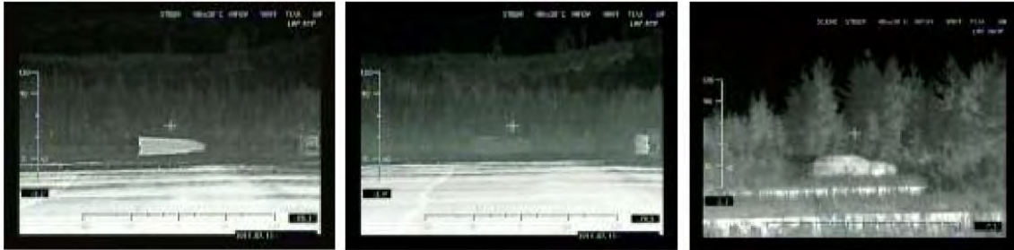
Figure 18. The center picture demonstrates the vast reduction in the vehicle's thermal and infrared red signature with the employment of Signature Management Measures in the form of Thermo-Variable tiles (from Armada 2013).
