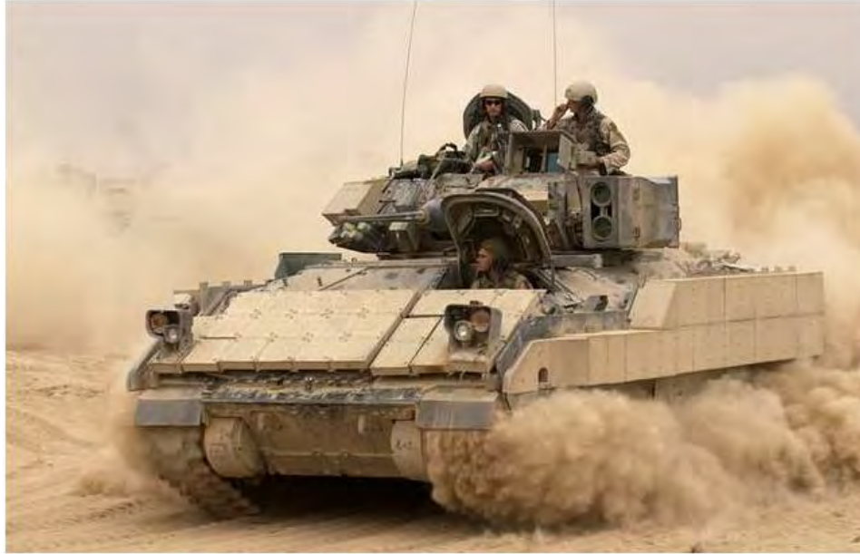
Figure 16. M2 Bradley AFV Mounted with ERA Cassettes (from Osborn 2007).
