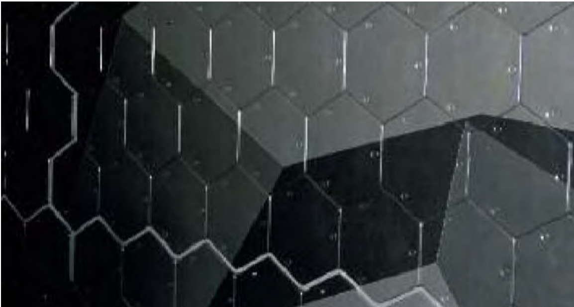
Figure 17. Thermo-Variable Tiles Mounted on a Combat Vehicle (CV) – 90 (from Armada 2013).
