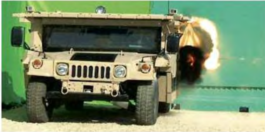
Figure 15. Trophy APS Intercepting an Incoming Hostile Projectile (from Armada 2013).
