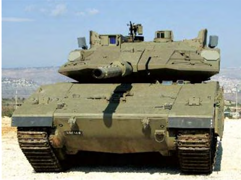
Figure 25. APS (Trophy) mounted on a Merkava Mk 3 of the Israel Defense Forces (from Armada 2013).
