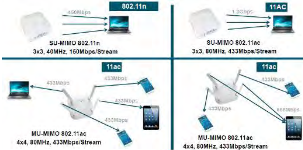
Figure 15. Different MIMO configurations used by 802.11n and ac.
