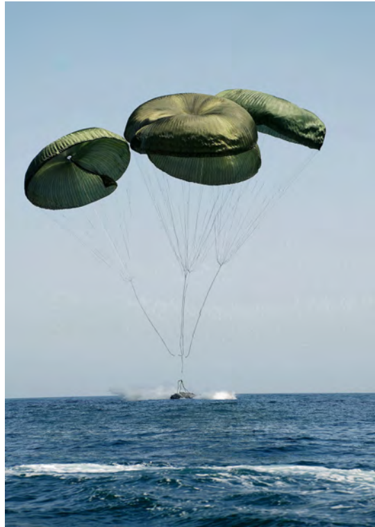
Figure 2.5: Maritime Craft Air Delivery System (MCADS). A Naval Special Warfare 11-meter Rigid Inflatable Boat is delivered during exercise FLEXIBLE LEADER 07. U.S. Navy photograph.
