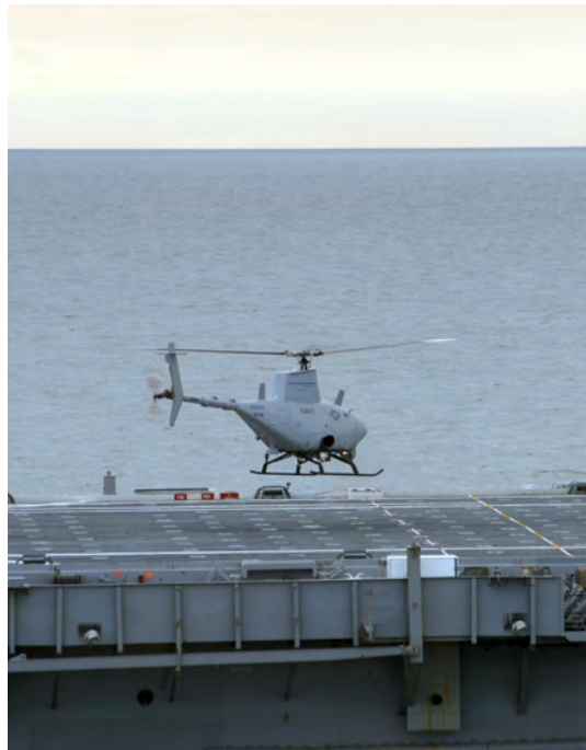
Figure 2.9: RQ-8A Fire Scout UAS prepares for autonomous landing. The vehicle hovers above the deck before landing autonomously aboard the amphibious transport dock ship USS Nashville (LPD-13). U.S. Navy photograph, 17 January 2006.
