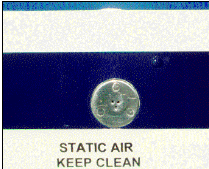
Figure 10-7. Standard Static Port Installation on Side of Fuselage
