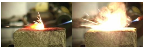
Figure 4. Combustion experiments performed on a) 22.5 wt.% nano-Al/PMMA and b) 22.5 wt.% nano-Al/ Zonyl ® TM fluoropolymer composite material.
