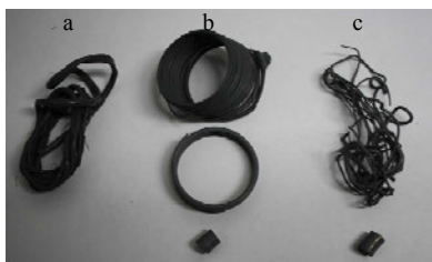
Figure 2. Picture displaying the extruded nano-Al/ Zonyl ® TM fluoropolymer composite at a) less than 20 wt.%, b) 22.5 wt.% and c) 34.5 wt% nano-Al content.
