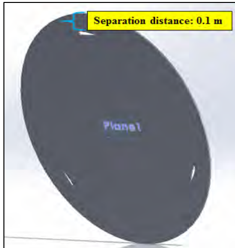
Figure 15. Rotor model created in Solidworks with NACA0018 blade profile.
