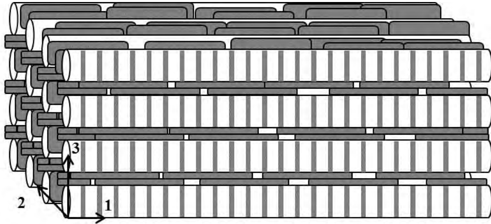
Figure 12. Three-dimensional fiber array. Dark rectangles represent HA crystals while the rod structures represent fibrils.
