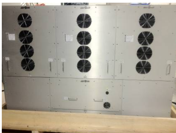
Figure 4-11: Schematic drawing and image of 100kW LFP power supply; up to 3 independent channels
