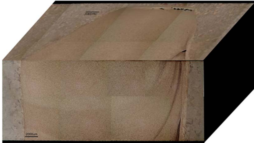
Figure 21. Plan view 12.7mm weld cross section highlighting material flow about the defect.
