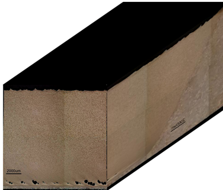
Figure 22. Longitudinal view of 12.7mm cross-section showing defect formation at the bottom of the stir zone. Defects appear to be forming and reconsolidating through the length of the weld.
