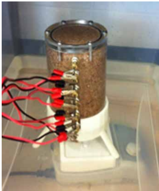
Figure C6-16: DEC in reservoir containing tracer-spiked water.
