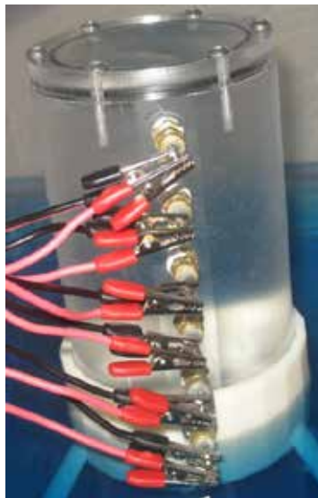
Figure C6-10: Open column experiment where only water is placed into column.
