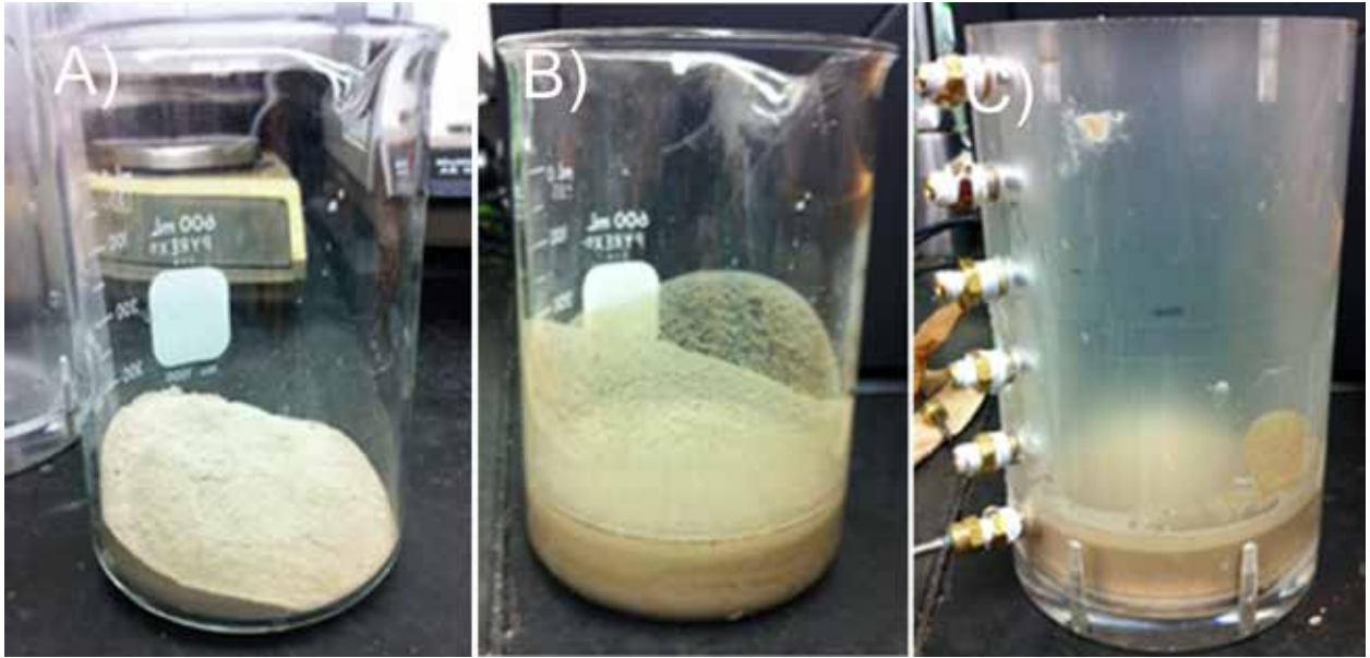
Figure C6-15: (A) FEW silt sample placed in beaker (B) water added to make saturated slurry (C) wet packing silt slurry into DEC.
