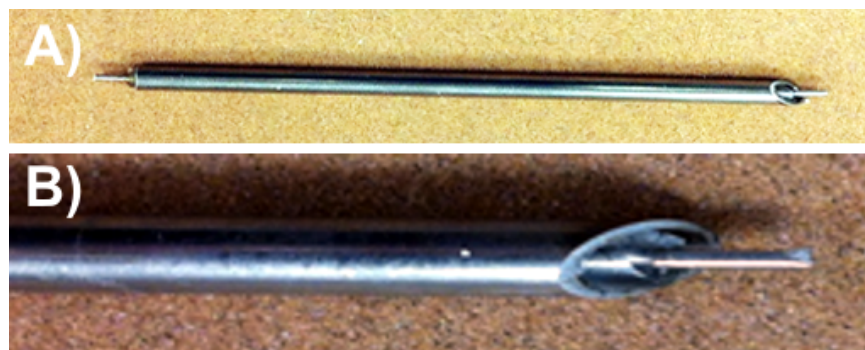
Figure C6-13: (A) Electrical conductivity probes (B) plastic tubing separates outer stainless steel needle from inner needle.
