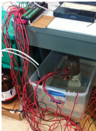
Figure C6-17: DEC in reservoir and attached to datalogger.
