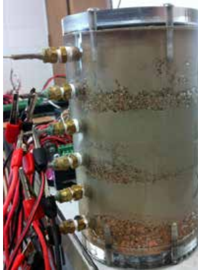
Figure C6-19: Layered column with alternating sand and silt layers.
