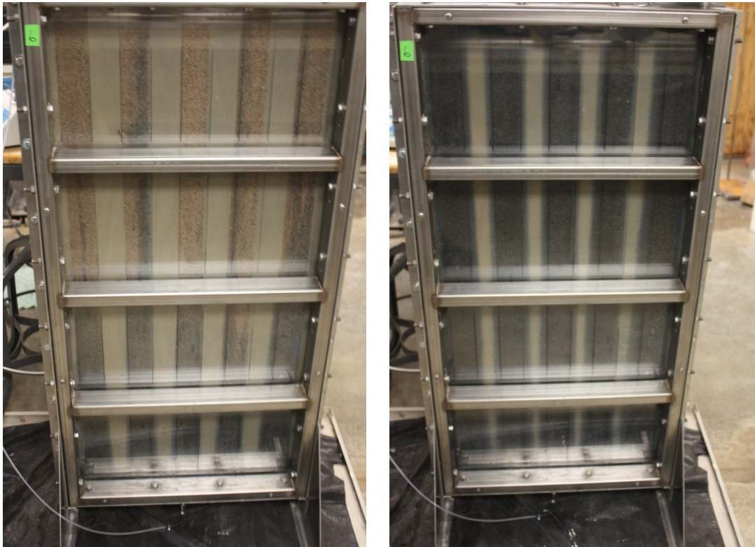
Figure 6-8: SRB treatment tank at the beginning (left) and end (right) of the 24-day treatment.
