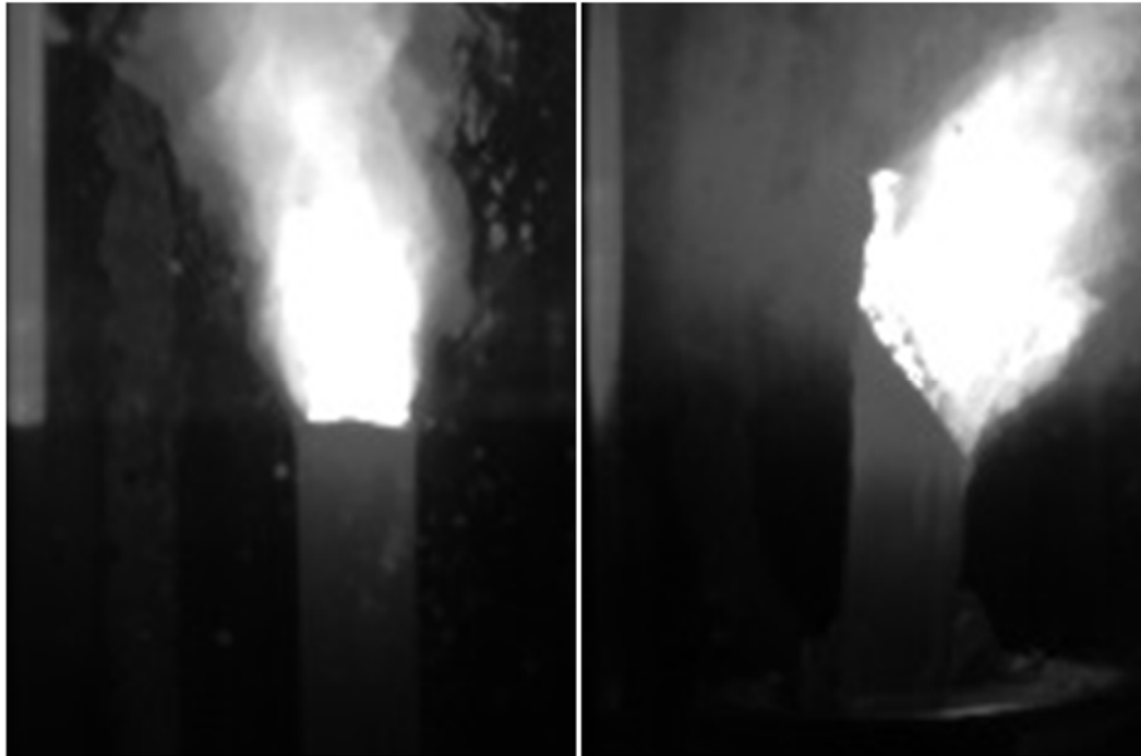
Fig. 2 Results obtained with configuration no. 1 test article: 1) foil-less section (left), 2) section with 0.001-inch-thick Al foil attached to right side (right)
