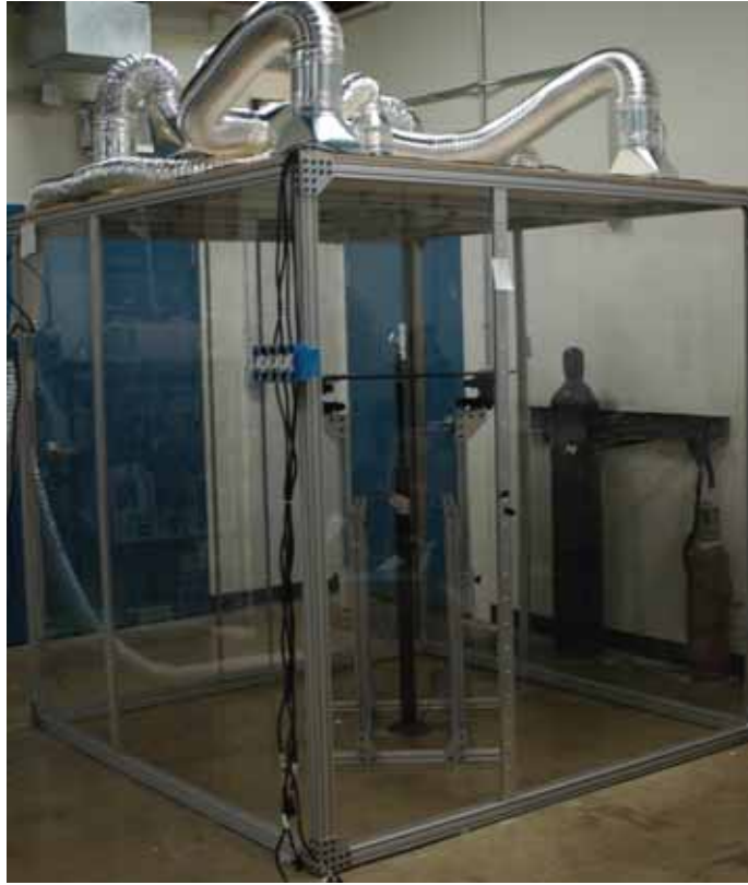
Figure 2.5: The dust chamber in which the flow experiments are performed.
