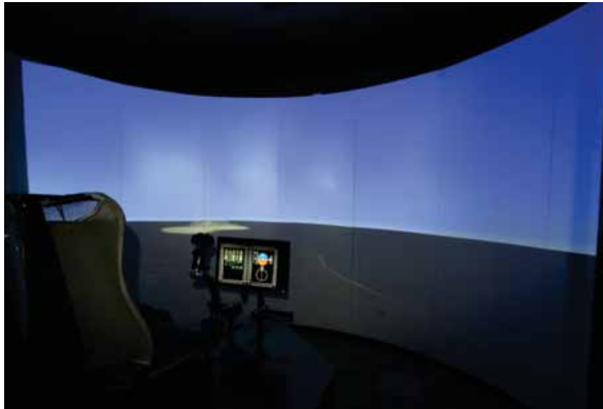
Figure 3.7: Set-up of ART's flight simulator integrated with brownout plugin.
