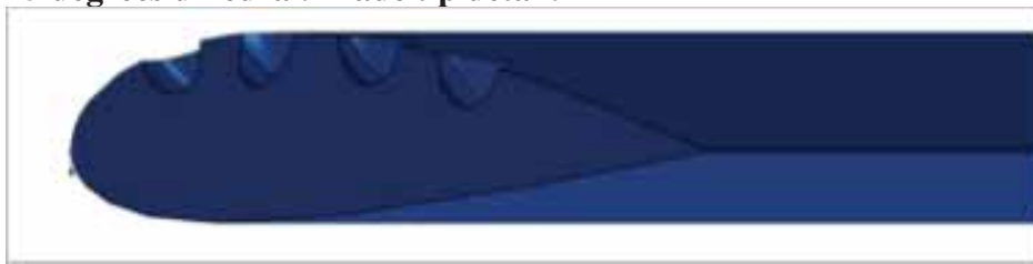
Figure 3.25: A modification made by relocating the blowing orifices at the upper edge and oriented at 45 degrees dihedral. Blade tip detail.
