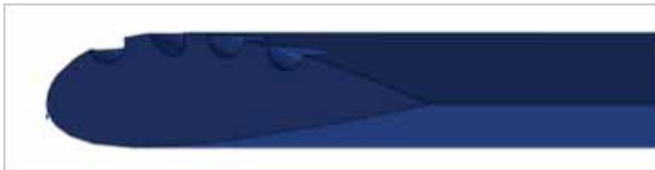
Figure 3.26: A modification made by increasing the dihedral angle to 60 degrees. Blade tip detail.
