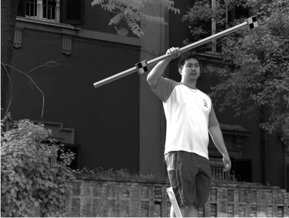
Figure 1 (20110511_cam3_000002.jpg): Image for midge swarm extrinsic parameter calibration showing the new calibration target.
