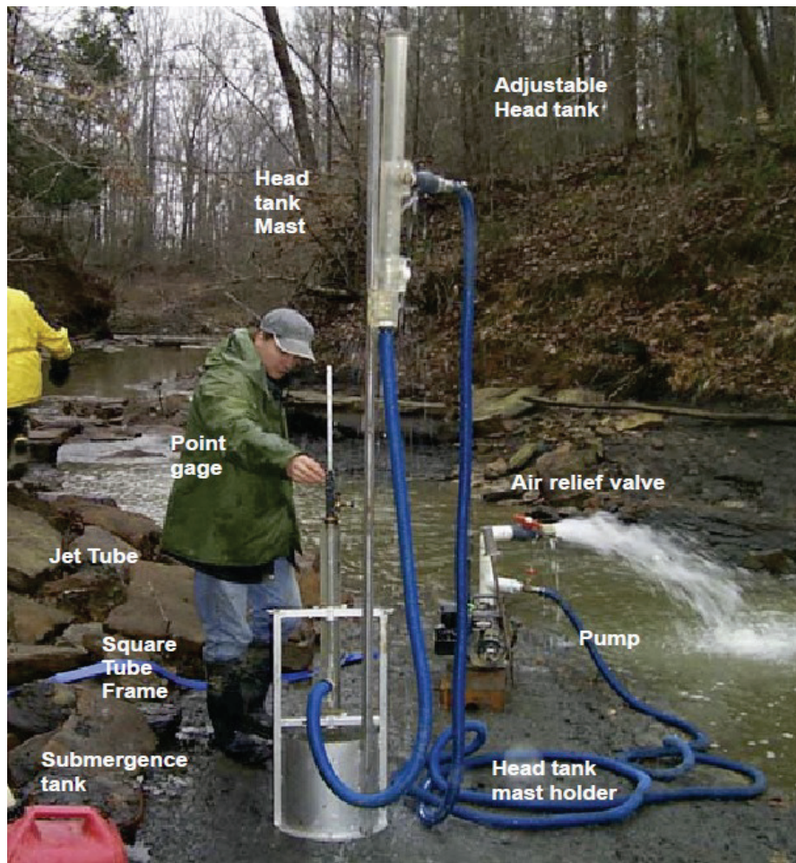
Figure 1. Original JET apparatus using constant water head system (Hanson and Cook 2004, reprinted with permission).
