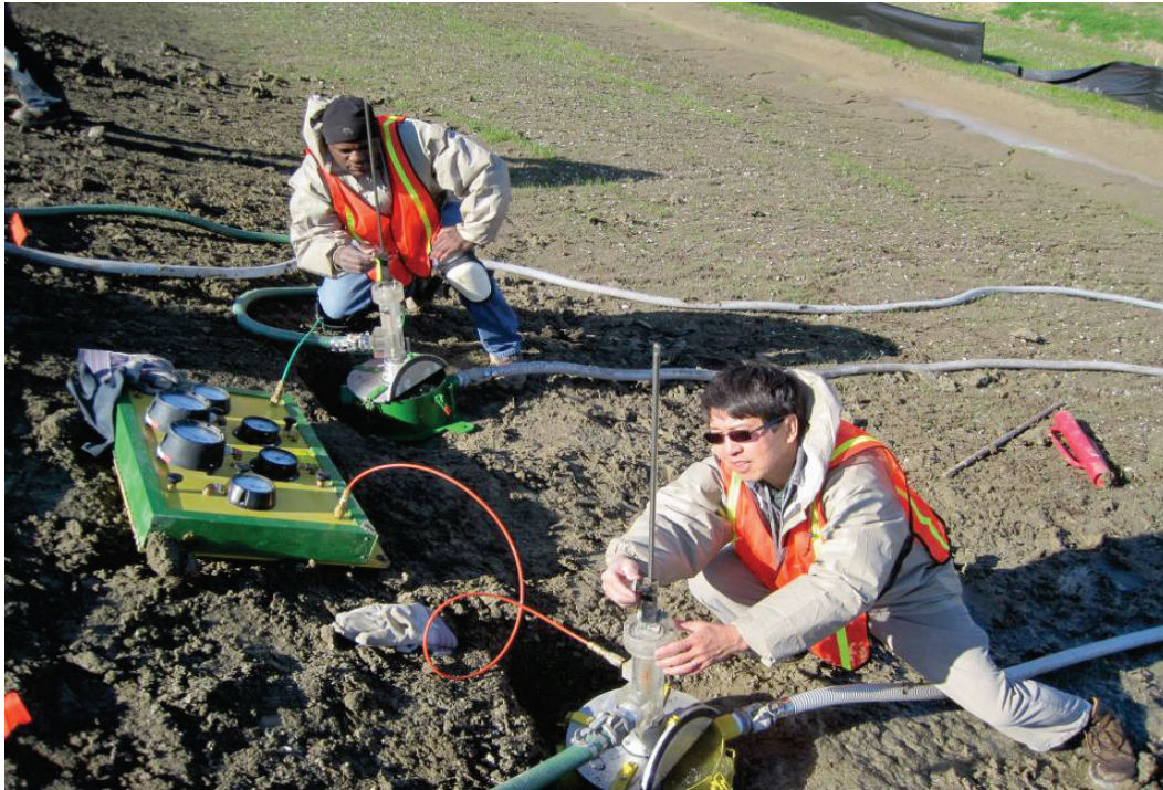
Figure 12. Engineers from ERDC performing field JET on fly-ash/bed-ash-treated segment.
