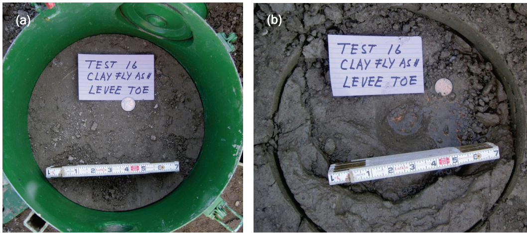
Figure B15. Test 16 (a) before and (b) after a field JET was performed.
