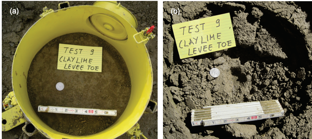
Figure C1. Test 9 (a) before and (b) after a field JET was performed.
