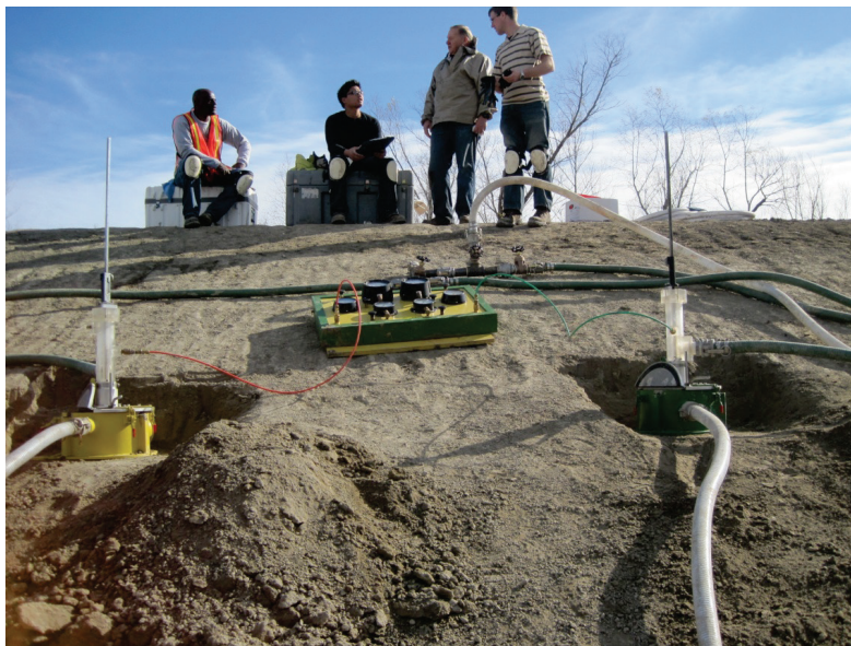
Figure 2. NSL-modified JET apparatus using an alternate water pressure source.
