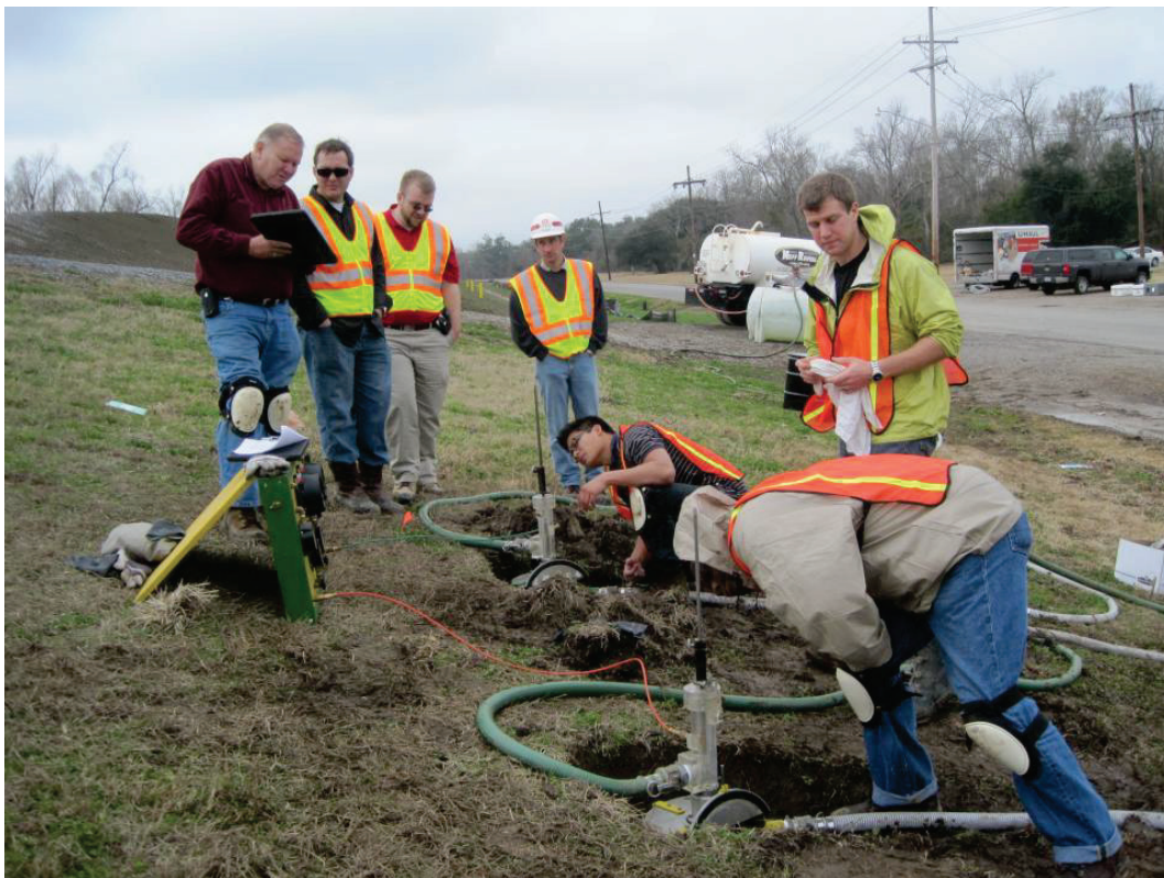
Figure 7. The ERDC team performing an erosion field JET on the untreated clay segment.
