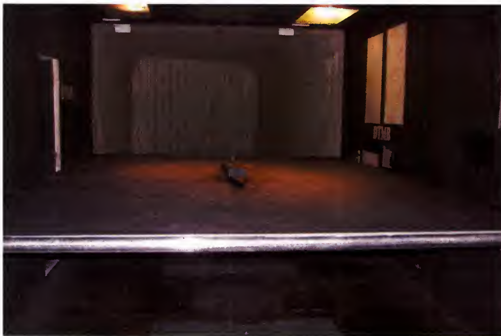
Figure 5. SWT test section with ground board and SFS2 model installed.
