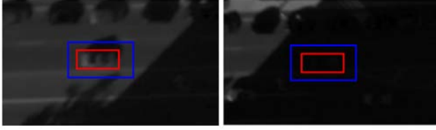
Fig. 6. Pixels within the red rectangle form the foreground (Fg) distribution, pixels between the red and blue rectangles form the background (Bg) distribution. Left: High VR when Fg and Bg regions have different distributions. Right: Low VR when Fg and Bg regions have similar distributions.
