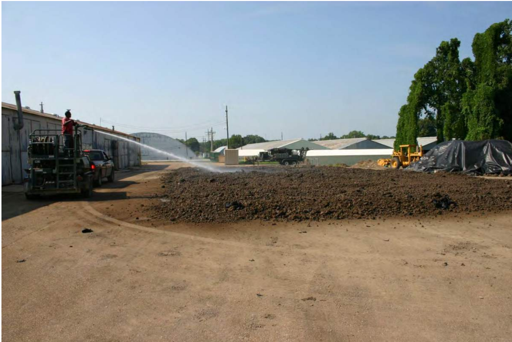
Figure 10. Addition of water to adjust moisture content.
