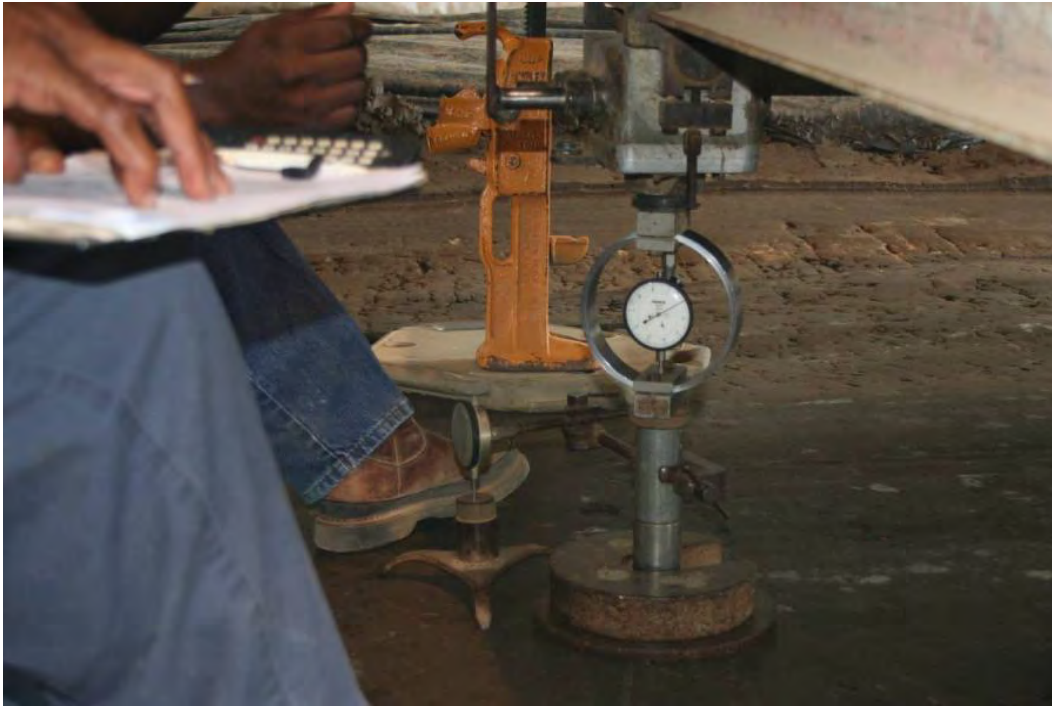
Figure 14. Field CBR test.
