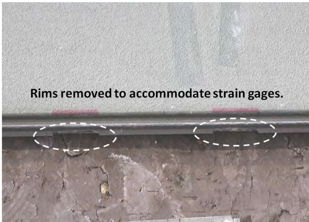
Figure 19. Modification to male hinge of AM2 panel.
