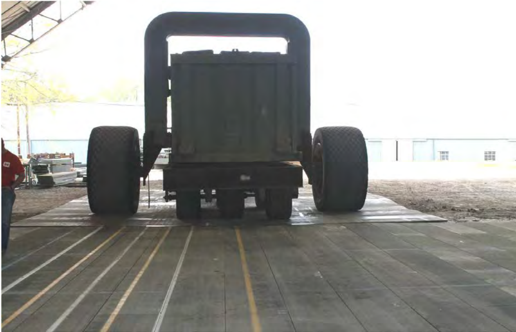
Figure 26. C-17 test load cart.
