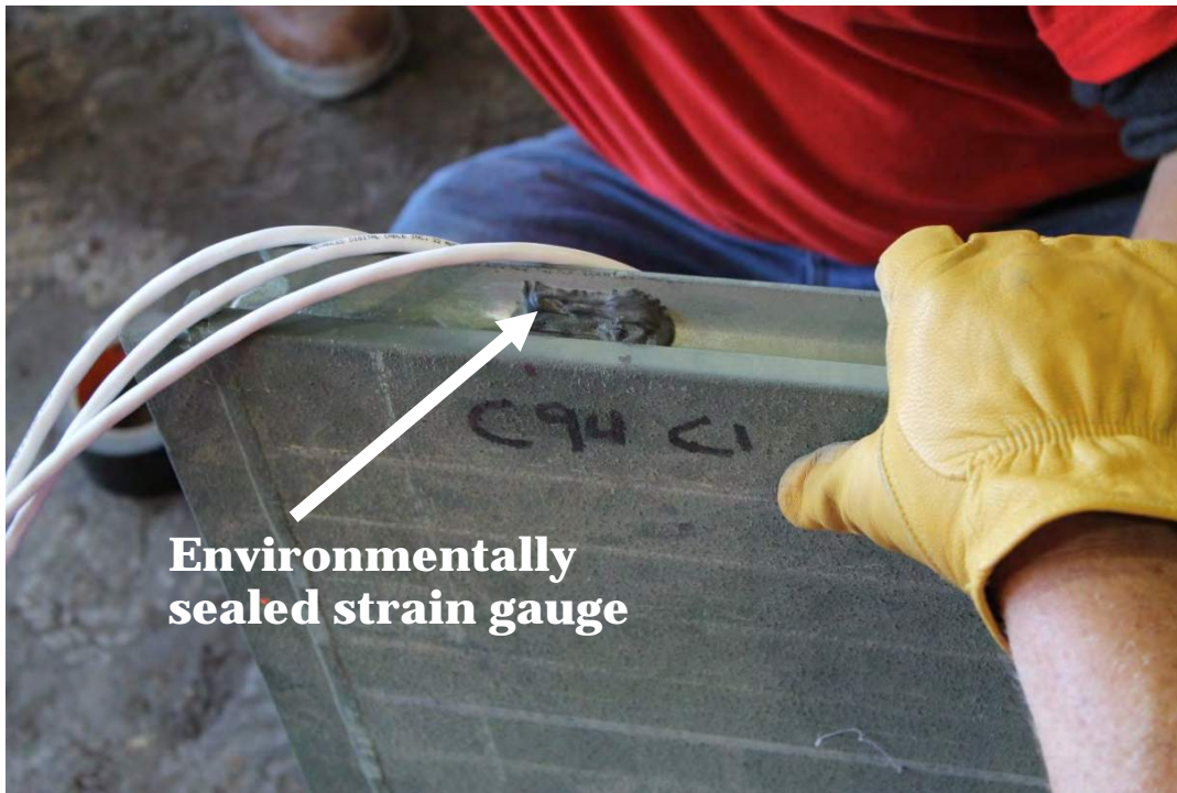
Figure 18. Typical strain gauge placement on female hinge connector of AM2 panel.
