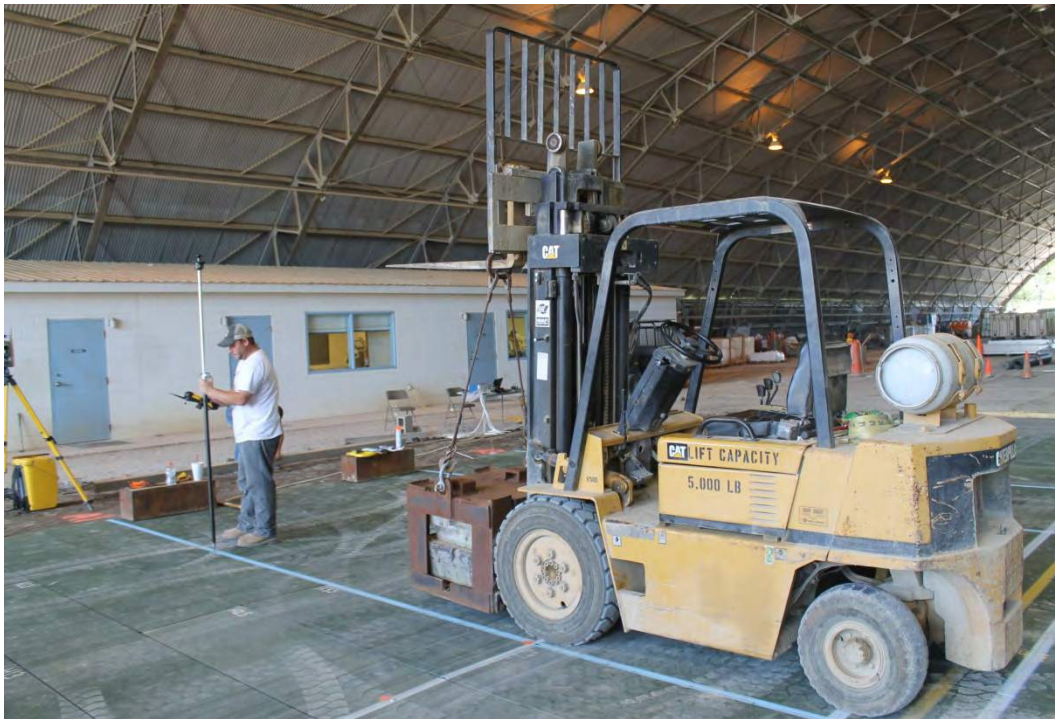
Figure 30. Typical survey of loaded cross section.
