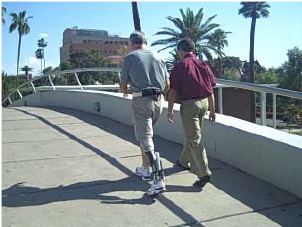
Figure 2: Subject is walking on an inclined surface where the angle is constantly changing. Two small batteries are carried at the waist.
