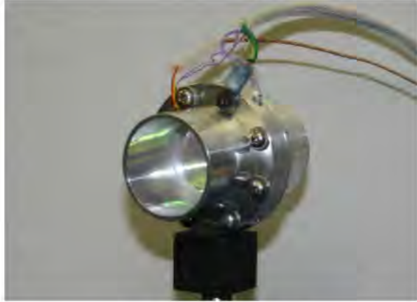
Figure 9. Temperature-controlled oven for use inside the spectrophotometer.
