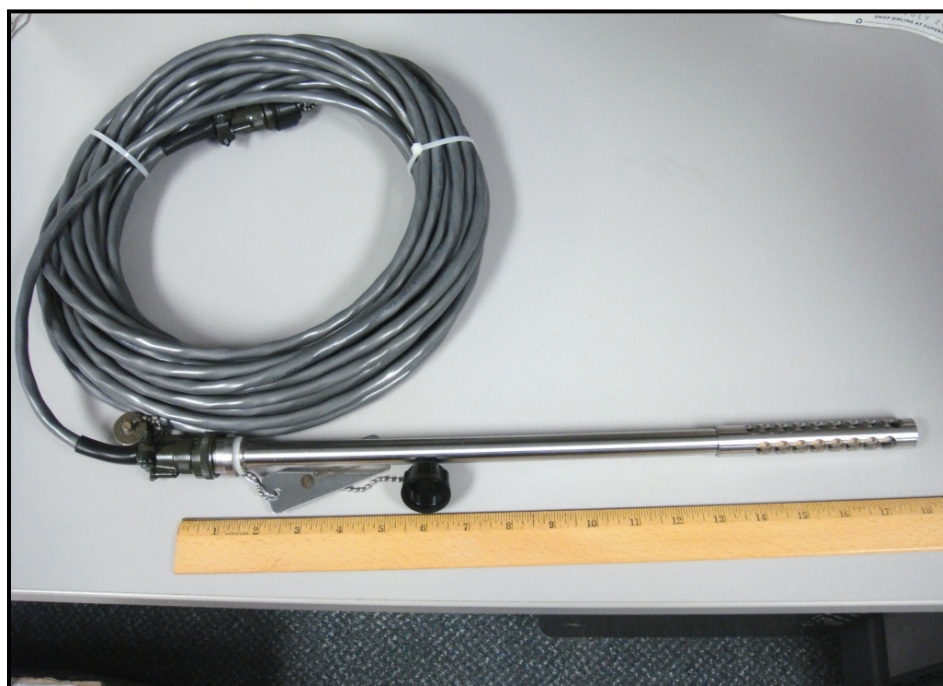
Figure 2-1. Typical ER probe used for this project.
