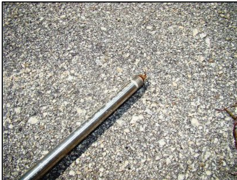
Figure 3-1. Damaged control probe. Note missing probe tip.
