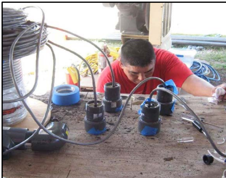
Figure 2-3. Encapsulation of probe connectors. Not visible are the probe bodies extending through holes in the work surface
