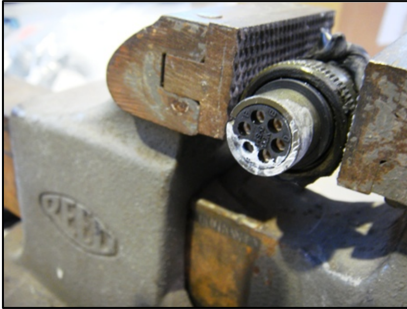
Figure 3-2. Corrosion of ER Probe Connector.
