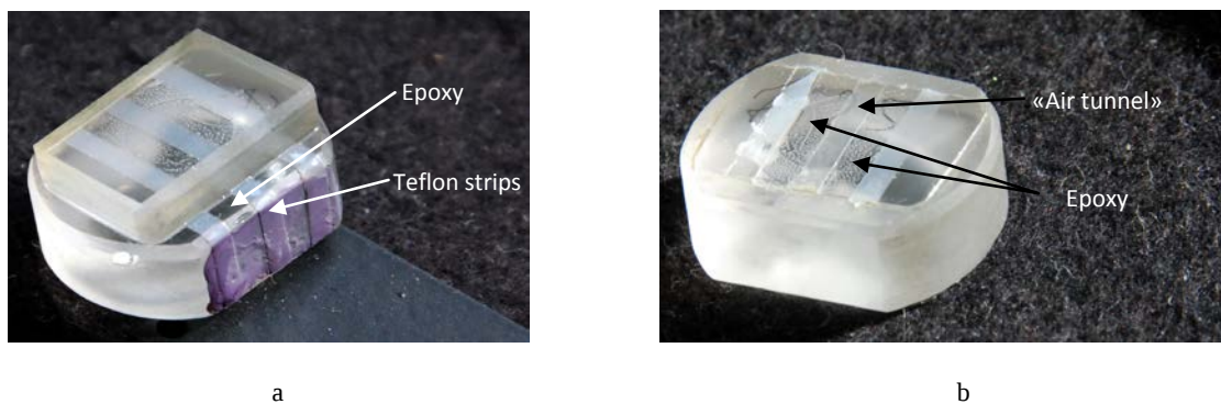
Fig. 2.4.2. Fabrication of a defected specimen with an “air tunnel” type of a defect. a – the plate of fused quartz is bonded to a block of the same material with epoxy resin; its thickness is 50\ \mu\text{m} and is determined by the thickness of Teflon strips. b – the plate is ground and polished down to the thickness of 90\ \mu\text{m} and the strips are pulled out.
