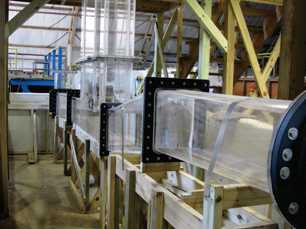
Figure 7. Dry bed view of the 1:15-scale model looking downstream.
