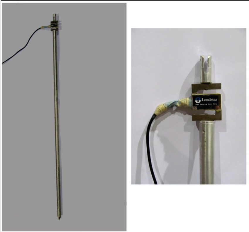
Figure 11. Load cell and strut prior to assembly.
