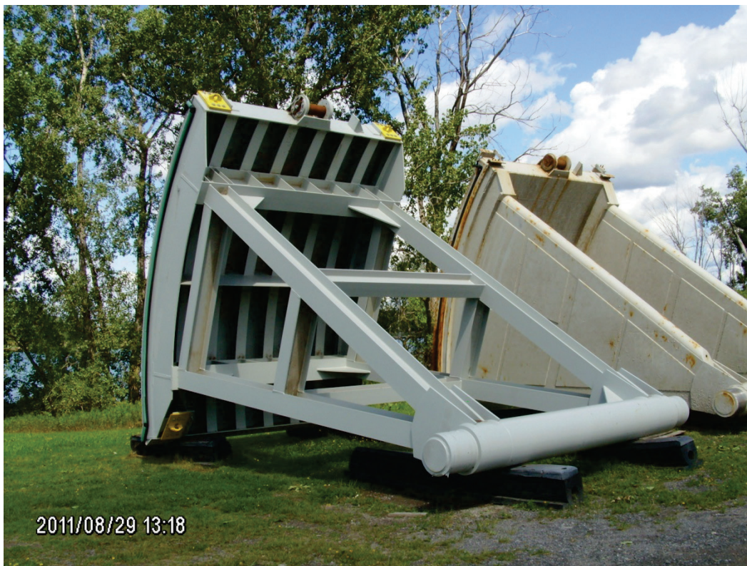
Figure 4. Prototype valves, new vertical-frame valve in foreground and used double-skin-plate valve in background.
