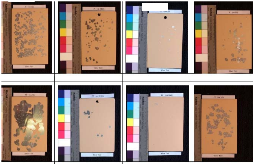
Fig. 12 Picklex on (from left to right) Al, CRS, galvanized, and stainless steel (53030 top, 53022 bottom)
