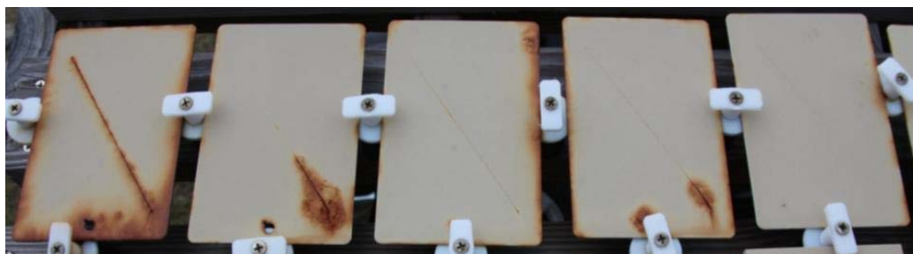
Fig. 37 Bonderite 7400 on CRS primed with MIL-DTL-53022 after 2 years
