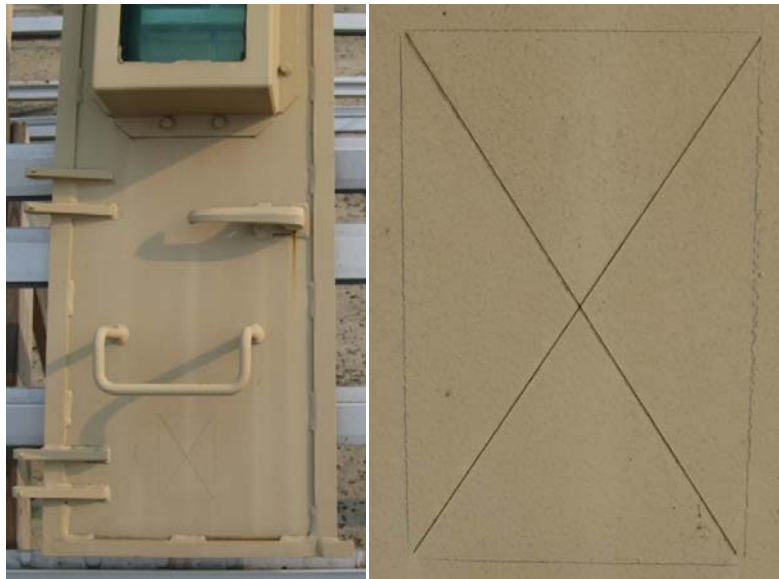
Fig. 47 MRAP door with Oxsilan 9810/2 after 2 years with close-up of scribed area
