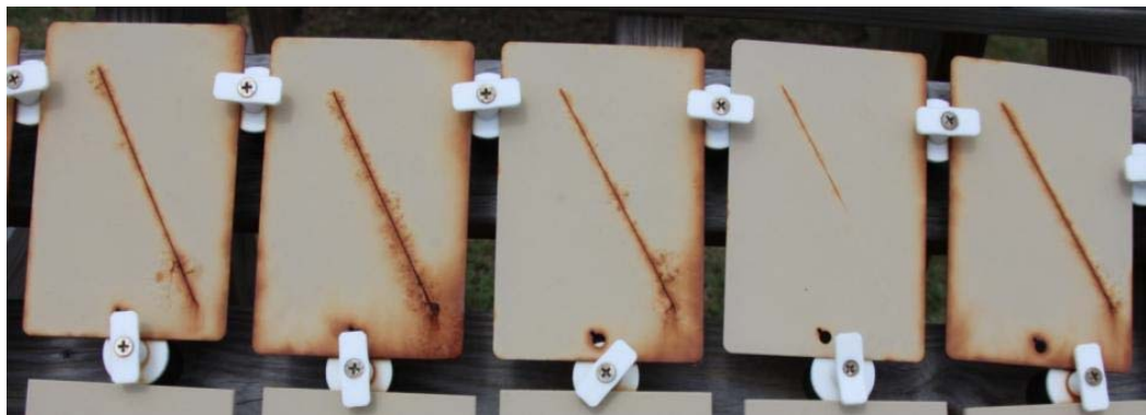
Fig. 39 DOD-P-15328 on CRS primed with MIL-DTL-53022 after 2 years
