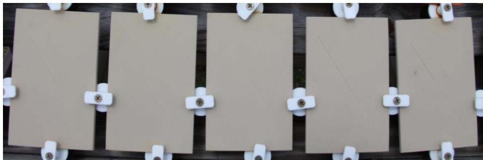
Fig. 44 DOD-P-15328 on Al primed with MIL-DTL-53022 after 2 years
