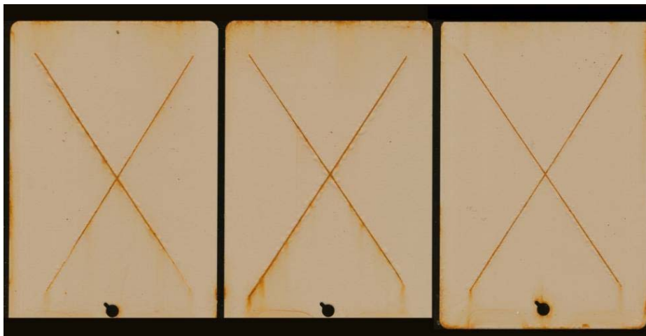
Fig. 20 Ecosil 5-1 on CRS primed with MIL-DTL-53022 after 80 cycles
