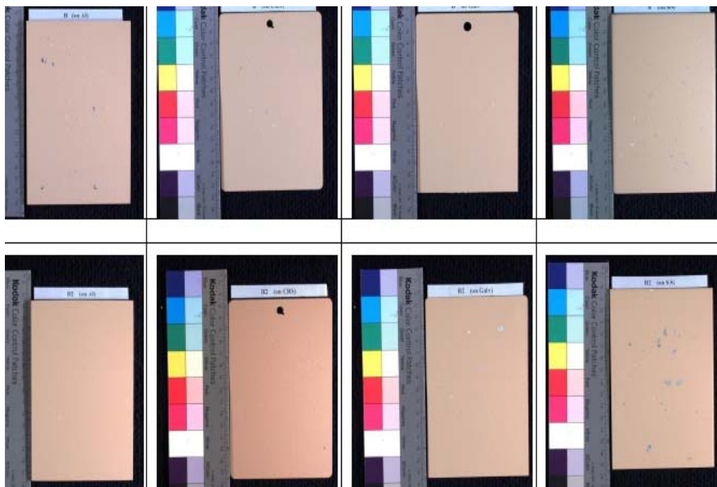
Fig. 9 Bonderite 7400 on (from left to right) Al, CRS, galvanized, and stainless steel (53030 top, 53022 bottom)
