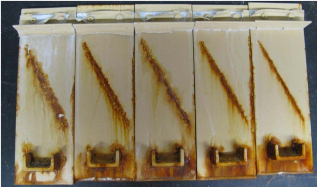
Fig. 33 Ecosil 5-1 on multimetal panels primed with MIL-DTL-53022 after 80 cycles
