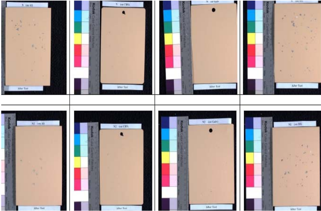
Fig. 11 DOD-P-15328 wash primer on (from left to right) Al, CRS, galvanized, and stainless steel (53030 top, 53022 bottom)
