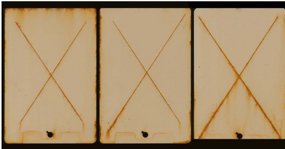
Fig. 19 Bonderite 7400 on CRS primed with MIL-DTL-53030 after 80 cycles
