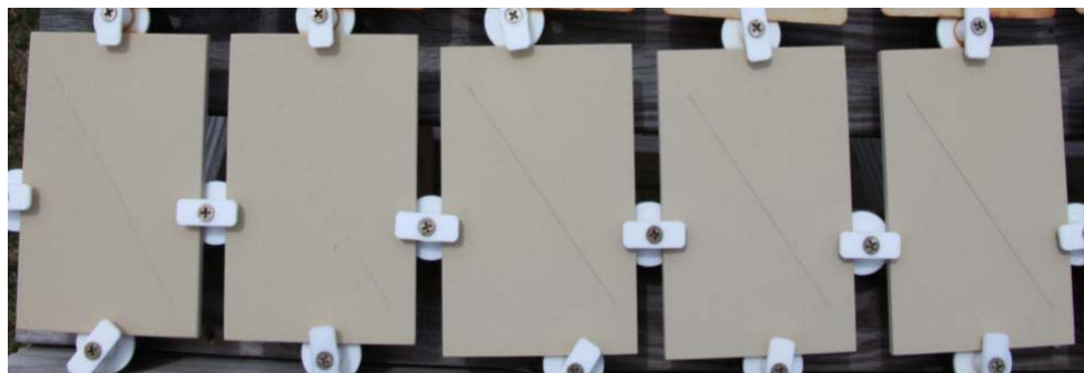
Fig. 45 DOD-P-15328 on Al primed with MIL-DTL-53030 after 2 years
