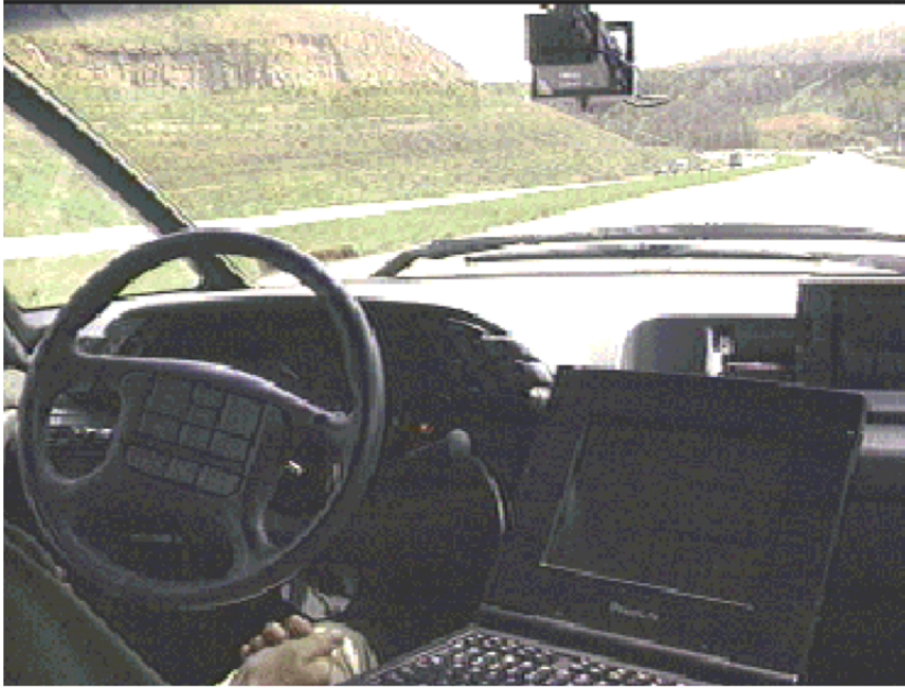
Figure 2: Pomerleau’s Autonomous Land Vehicle in a Neural Network system at work driving the Carnegie Mellon NAVLAB vehicle. Used with permission.
