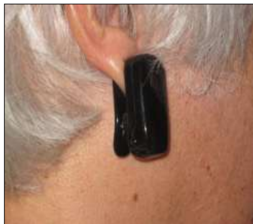
Exhibit 5. Wireless Pulse Sensor
