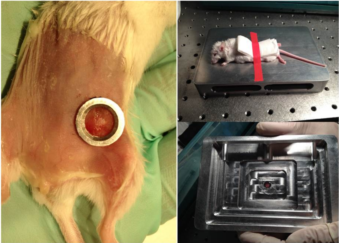
Figure 5: New fixturing for intravital FLIM imaging through a rodent mammary imaging window. Stage is raised to accommodate tall 20xW objective.
