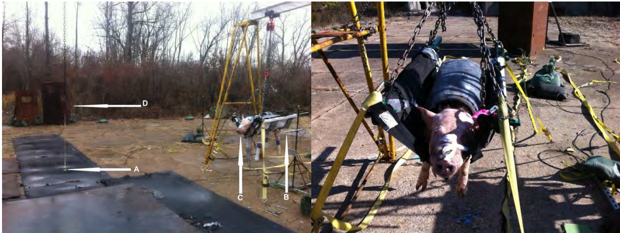
Figure 2. Blast experiment setting. The left photograph shows the anesthetized swine placed in a steel-covered sling hanging from a metal beam which is anchored to the ground. The arrow at "A" points to the C4 charge. The distance of the C4 explosive to the test animal was adjusted to vary the IOP. Arrow B shows the pencil pressure sensor used to record the incident pressure. Arrow C shows the head of the test animal directly facing the oncoming blast wave front. Arrow D shows the location of high-speed cameras and blast shielding. The right photograph shows the swine in a metal harness anchored to the ground and covered with a foam-lined lead shield over the torso.
