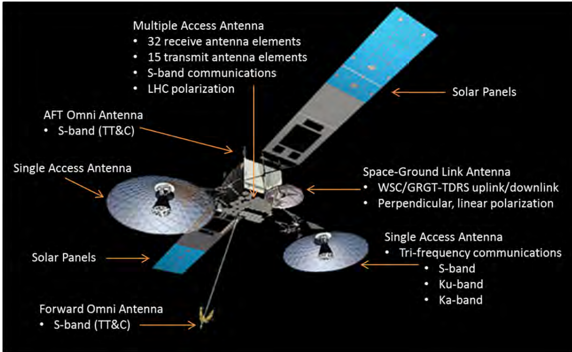
Figure 2. Third Generation TDRS Overview (from [4])
